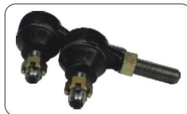
A tie rod is a slender structural rod in the steering mechanism of a vehicle. The tie rod ends are flexible couplings
